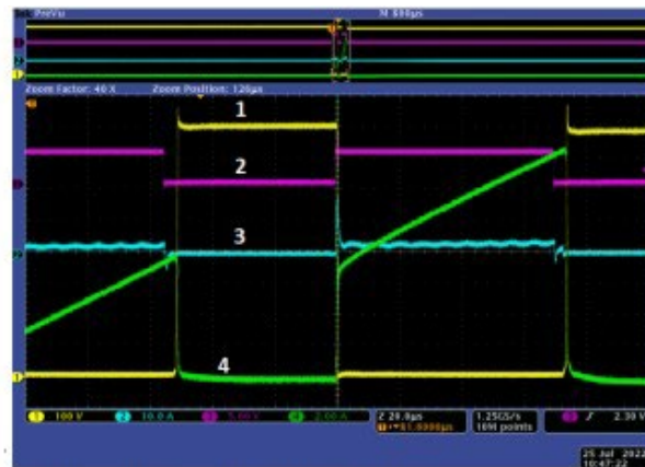
1: V_{CE} , 2: Control Sig., 3: I_B and 4: I_E
