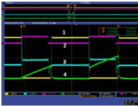
1: V_{CE} , 2: Control Sig., 3: I_B and 4: I_E
