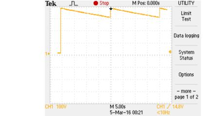
Figure 1: PCS DC Port Precharge Output Waveform, relative to Earth Ground
